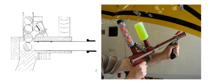
Figures 4: The barrel is returned to the neutral position, capturing the sphere as it moves aft. The index finger on the forward hand should be used to ensure that the barrel has seated. The sphere is now ready to be launched by momentarily pulling the trigger lever aft, releasing a burst of compressed gas behind the sphere(s) and propelling it (them) out of the barrel.
