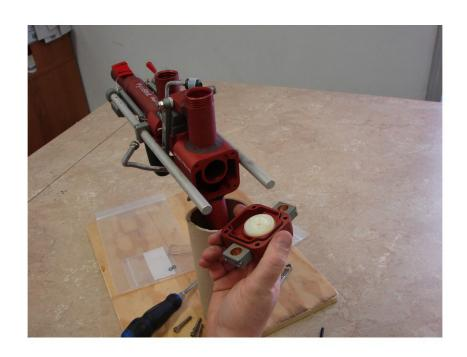
Insert 1-½" length by 3/8" diameter polyurethane rods into the handle and receiver to reduce the shot tank volume. The maximum number of rods is 26, sixteen in the handle and ten in the receiver. It is a little tricky getting the 16 rods into the handle, and requires a bit of patience and manipulation. The ten in the receiver are straightforward, as they are inserted straight in around the barrel circumference.
