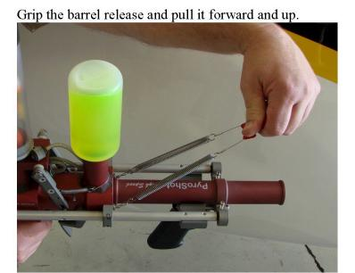
Pull the barrel straight out of the receiver.
