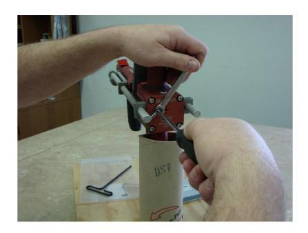
Gently bend the air tube out of the way of the valve housing, then remove the four cap screws that retain the valve housing, using a 5/32 allen wrench. The valve housing can now be removed by carefully sliding it directly aft until the slide rod bushings clear the slide rods.
