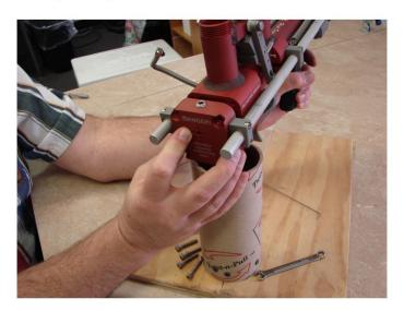
In addition to a 5/32 hex wrench, the volume reduction kit (or "stuff kit") includes a wire hook tool for extracting the rods from the receiver and handle and several spare O-rings.
