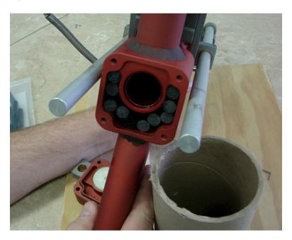
Each length of rod displaces 0.165 cubic inches, so you can calculate the amount of shot tank volume reduction. That is approximately 1 cid per 6 pieces or a bit more than 4 cid for all 26 pieces supplied.
