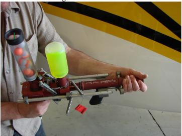
Hold a charged barrel muzzle up and away from the body. Charged rounds will fall from the barrel as they react.
