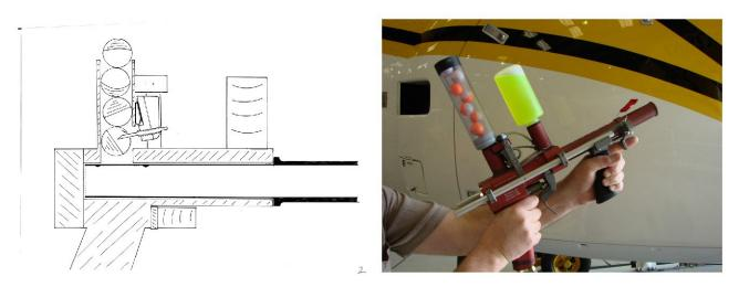
Figures 3: The injector mechanism is moved forward to the neutral position, extracting the needle from the sphere. The barrel is then moved forward in the receiver, allowing the injected sphere to drop into the receiver. (If two spheres are to be launched, a second sphere may be injected and loaded at this point. The chamber is designed for two rounds.)
