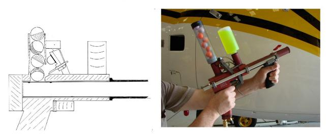
Figures 2: As the injector mechanism is moved aft, the needle pierces the bottom-most sphere and then the pump presses against the surface of the feed tube, injecting the sphere with ethylene glycol. The sphere is now "charged" and will ignite in approximately twenty seconds (or more, depending on ambient temperature).
