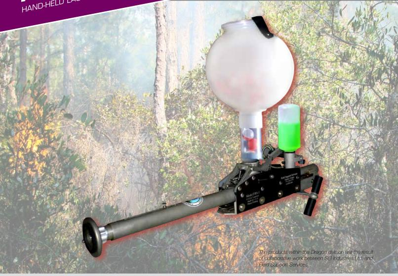
The Pyroshot is one of the newest tools to support ground fire ignition during burn operations. The single-shot Pyroshot is an incendiary plastic sphere dispenser that can best be described as a hand-held, spring-powered gun. Costing far less than traditional flare guns, the Pyroshot can launch spheres upwards of 75 ft. (23m) and is a lightweight tool that uses SEI's Dragon Eggs.
