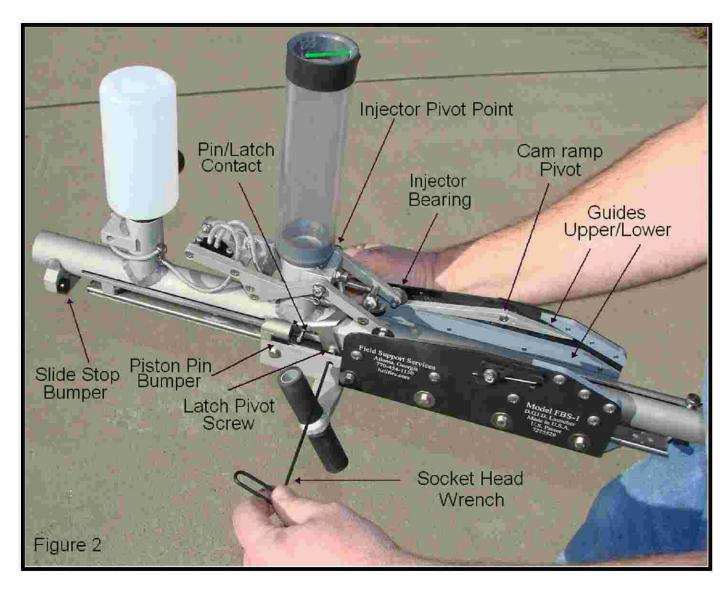
6. Lubricate as required.... One drop of light machine oil on each latch pivot point, injector pivot point, injector bearing (including the large area washer) and cam ramp pivot point. Spread a small amount of
