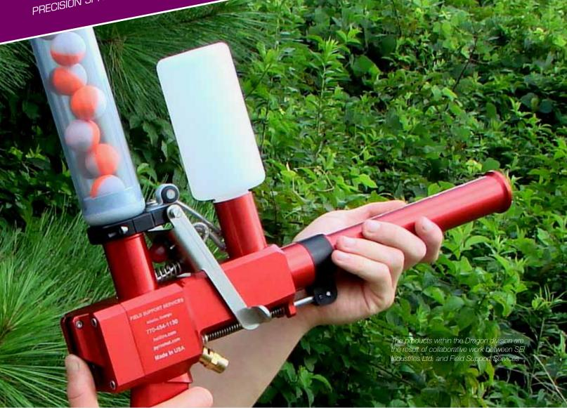
The Pyroshot 'High Speed' is a gas-propelled, triggeractivated Dragon Egg hand-launcher. The Pyroshot HS uses a 5 lbs. CO<sub>2</sub> beverage bottle (or a 20 ounce mini-bottle carried on the belt) to easily launch Dragon Eggs 320 ft.
