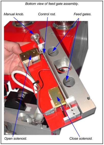
To open the gates, the open solenoid energizes and pulls out the locking pin. An opening spring on the feed control rod causes it to move outwards into the fully open position. The open solenoid then de-energizes.
