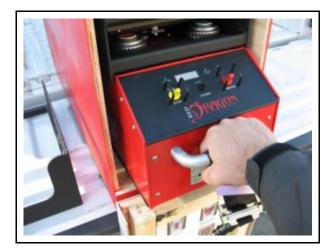
• Remove the hopper from the machine by grasping the hopper lock handle and pulling up.
