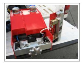
• Unlock the feed gate control rod by lifting up on the open solenoid plunger with a slotted screwdriver. The feed gate control rod should spring open.
