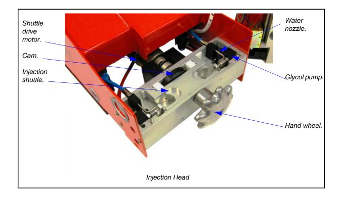
The injection head is the heart of the Red Dragon Dispenser. It is here that the Dragon Eggs are pierced by a hollow needle, injected with a controlled amount of glycol and then ejected from the machine.
