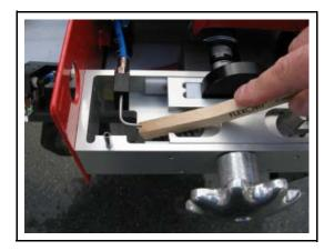
• Clean the injection head and shuttle using a cloth and a citrus-based cleaner/degreaser such as Simple Green all purpose cleaner. If an appropriate cleaner is not available, water can be used (with caution).
