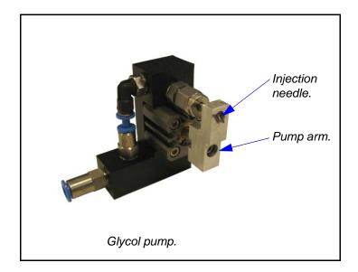
If the machine is operated until the glycol pumps drain the tank, the pumps will lose their prime. The pump assemblies may be removed from the injection head and re-primed by squeezing the pump arm repeatedly until glycol flows from the injection needle. Each pump assembly is secured to the injection head by two captive screws.
