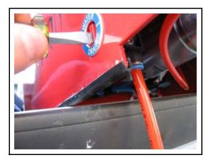
• Remove the feed gate assembly.
