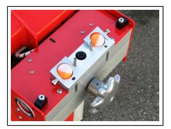
• Attach the tethered remote control to the control panel on the main body.
