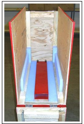
Place the main body of the dispenser into ٠ the crate with the control panel facing the open end of the crate.
