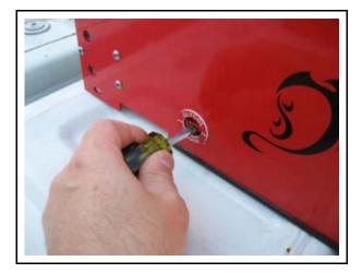
• Check/fill the water storage tank. Secure the filler/breather cap.
