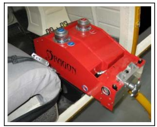
• Attach and secure the outlet chute, using a thumbnut and locking thumbnut on each screw.
