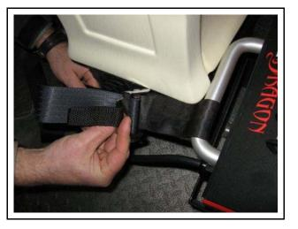
• Replace the hopper assembly onto the dispenser. Slide the dispenser as far forward as possible to provide leg-room between the dispenser and the rear seat. Ensure that the hopper lid opens freely. Tighten the belly strap snugly.
