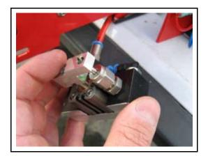
• Clean the injection shuttle and injection block.
