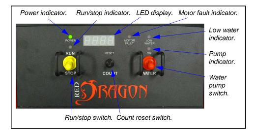
The control panel is the brains of the Red Dragon system. A single circuit board mounted beneath the main control panel contains the microprocessor and all additional components.
