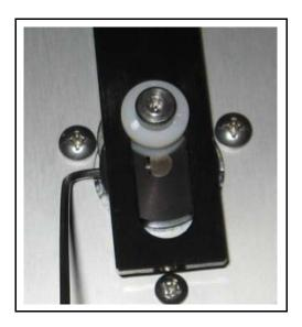
Replace the agitator mechanism into the hopper body and secure using four # 10-24 x 3/8 button head capscrews.
