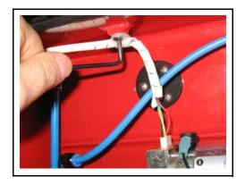
• Disconnect the motor wiring harness from the motor terminals.
