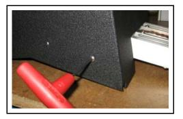
• Remove the agitator mechanism from the hopper body.
