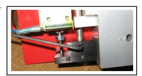
• Press on the close solenoid core to try to fully extend the pin on the close solenoid.
