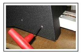
Remove the agitator mechanism from the hopper body
