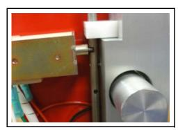
Replace the gate wiring harness wires onto the close solenoid terminals.
