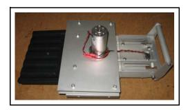
Remove the four # 4-40 x 3/8 screws which secure the wiring harness receptacle to the agitator assembly.
