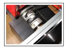
• Remove the two #10-32 x 1-1/4 socket head capscrews which secure the motor mount to the injection head.
