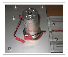
Align the motor shaft flat with the setscrew in the agitator cam and tighten the setscrew.
