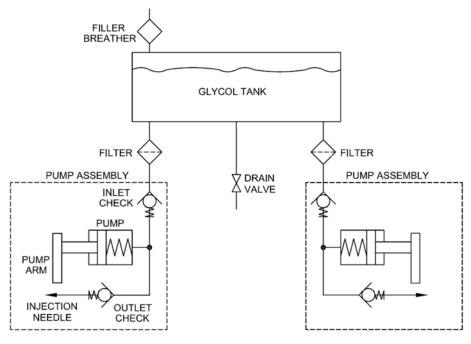
As the injection shuttle pushes a sphere towards the pump assembly, the tip of the injection needle pierces the sphere. Continued motion of the shuttle causes the sphere to press against the pump arm which compresses the piston. The inlet check valve is closed, preventing glycol from returning to the tank. As the fluid pressure in the pump cylinder rises, the outlet check valve opens, allowing the glycol in the pump cylinder to flow through the injection needle and into the sphere.
