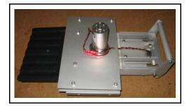
• Loosen the #8-32 setscrew which secures the agitator cam to the hopper motor shaft.
