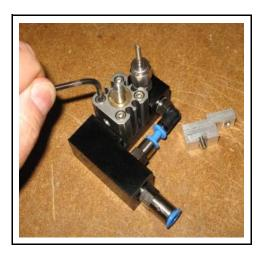
Replace the pump arm and secure to the pump piston using the 3mm x 1.5 socket head capscrews.
