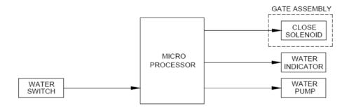
The dispenser is also equipped with a rechargeable battery. A built in charger system maintains charge on the battery whenever the unit is receiving power from an external power supply. When there is no external power supply, pressing the "WATER" switch connects the 12VDC emergency battery directly to the emergency water pump.
