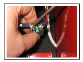
Cutaway the plug on the old wiring harness.
