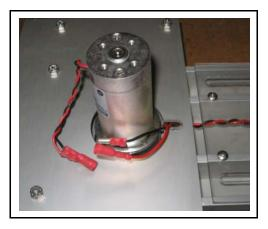
• Replace the agitator assembly into the hopper body and secure using four # 10-24 x 3/8 button head capscrews.
