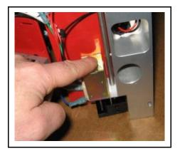
Adjust the position of the control rod so that the locking pin on the open solenoid aligns with the groove in the feed control rod.
