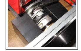
Remove the two #10-32 x 1-1/4 socket head capscrews which secure the motor mount to the injection head.
