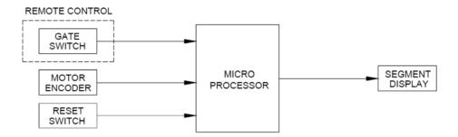
By pressing and holding the "COUNT RESET" switch, the sphere count can be reset to zero. By pressing the switch momentarily, the display can be toggled between normal display and a lifetime count of spheres indicated in thousands
