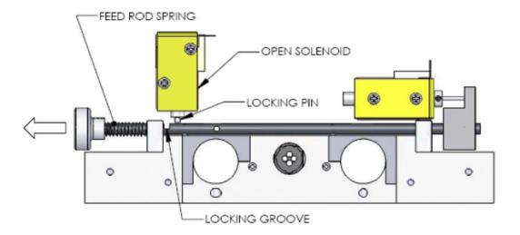
When the close solenoid is energized, it pushes the feed control rod inwards, causing the feed gates to block the flow of spheres through the passages. The spring loaded pin re-enters the groove in the feed control rod and locks the gates closed. In an emergency, the feed gate can be closed and locked by pushing the manual feed gate knob located on the end of the feed control rod.
