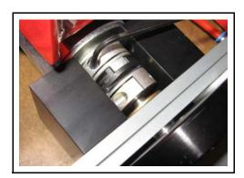
• If both hubs are turning, tighten the drive shaft hub.
