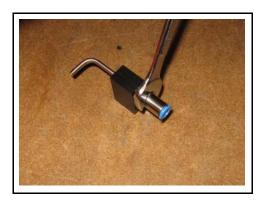
Blow out check valve with compressed air in the normal flow direction to clean the valve.
