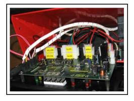
Replace the control panel and secure in place using four #10-24 x 3/8 button head capscrews.
