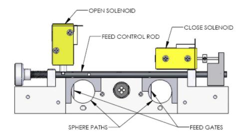
When the open solenoid is energized, it withdraws a spring loaded locking pin from the groove in the feed control rod. Once the feed control rod is unlocked, the feed rod spring forces the feed control rod to move outwards, unblocking the sphere paths.
