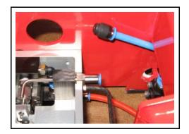
• Remove check valve from nozzle assembly
