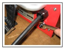
• Disconnect the power wiring harness from the main circuit breaker.
