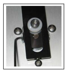
• Remove the two # 10-32 x 3/8 screws which secure the hopper motor to the hopper base.
