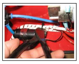
Attach the new pump wiring harness to the pump ensuring that the red lead is attached to the positive terminal
