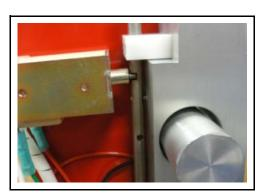
Replace the gate wiring harness wires onto the open solenoid terminals.
