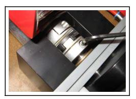
• If only the drive motor hub is turning, replace the coupling.
